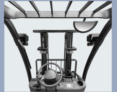
New designed mast and the large open steel roof provide super visibility, it also can reduce risk of accidents
