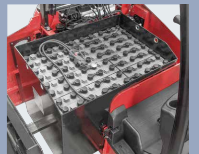
Side roll out the battery can provides the fast, simple and safe solution for the operator
